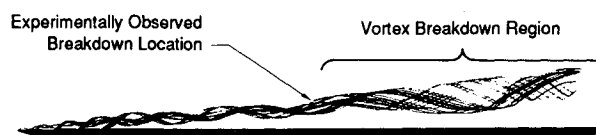
Fig. 5 Euler solution particle traces, 60-deg delta wing, angle of attack = 16 deg.
